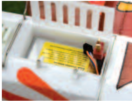
The battery compartment includes a plastic hatch cover.
